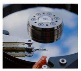
When gas systems operate, particularly inert gas systems, there is a very loud, high pitched noise on gas release. This can cause disruption and damage to Hard Disk Drives (HDD's) as it causes vibration to the head. As HDD's continue to get smaller and higher capacity this problem has increased over recent years with some high profile data outages caused by suppression systems.
