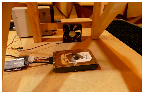
Figure 2: Photograph of the test set-up showing the HDD on an MDF board in the anechoic chamber at Michigan Technological University with the speakers placed 0.5 m above the HDD (left). The surface mount microphone, a fan used for cooling the HDD and the USB 3.0 cables used for performance test (right).
